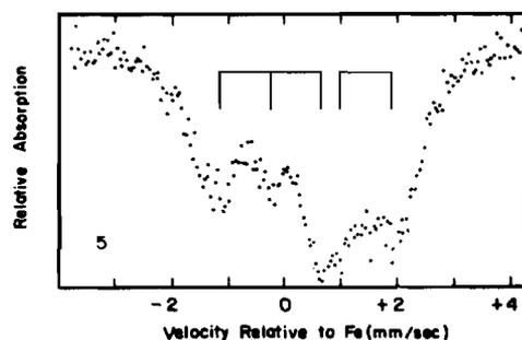
Figure 5. Magnetically Perturbed Mössbauer Spectrum of  $\text{Fe(salen)Cl} \cdot x\text{C}_5\text{H}_5\text{N}$ ,  $H_{\text{applied}} = 4.5$  kG.
