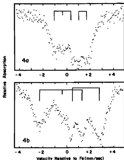
Figure 4a. Magnetically Perturbed Mössbauer Spectrum of  $\text{Fe(salen)Cl} \cdot x\text{C}_5\text{H}_5\text{N}$ ,  $H_{\text{applied}} = 4$  kG. 4b. Magnetically Perturbed Mössbauer Spectrum of  $\text{Fe(salen)Cl} \cdot x\text{C}_5\text{H}_5\text{N}$ ,  $H_{\text{applied}} = 8.8$  kG.
