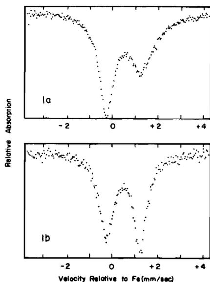
Figure 1a. Mössbauer Spectrum of Fe(salen)Cl · xC<sub>5</sub>H<sub>5</sub>N at 300°K. 1b. Mössbauer Spectrum of Fe(salen)Cl · xC<sub>5</sub>H<sub>5</sub>N at 4.2°K.
