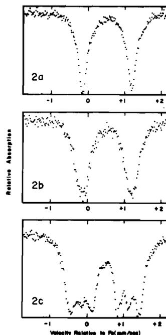
Figure 2a. Mössbauer Spectrum of [Fe(salen)Cl]<sub>2</sub> at 4.2°K. 2b. Magnetically Perturbed Mössbauer Spectrum of [Fe(salen)Cl]<sub>2</sub>,  $H_{\text{applied}} \approx 9$  kG. 2c. Magnetically Perturbed Mössbauer Spectrum of [Fe(salen)Cl]<sub>2</sub>,  $H_{\text{applied}} \approx 27$  kG.
