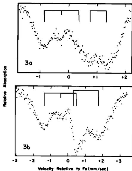
Figure 3a. Magnetically Perturbed Mössbauer Spectrum of  $\text{Fe(salen)Cl} \cdot x\text{CH}_3\text{NO}_2$ ,  $H_{\text{applied}} \approx 5.4$  kG. 3b. Magnetically Perturbed Mössbauer Spectrum of  $\text{Fe(salen)Cl} \cdot x\text{CH}_3\text{NO}_2$ ,  $H_{\text{applied}} = 10$  kG.
